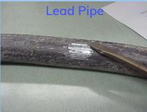
Scratch Test - if the pipe is soft and easily scraped and the becomes shiny, your pipe is lead.
