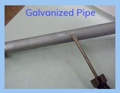
Scratch Test - if the scratched area remains gray, the service line is galvanized steel.
